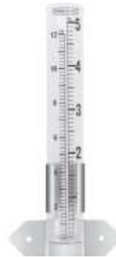
Figure 7. A rain gauge also works well for spreader calibration.
