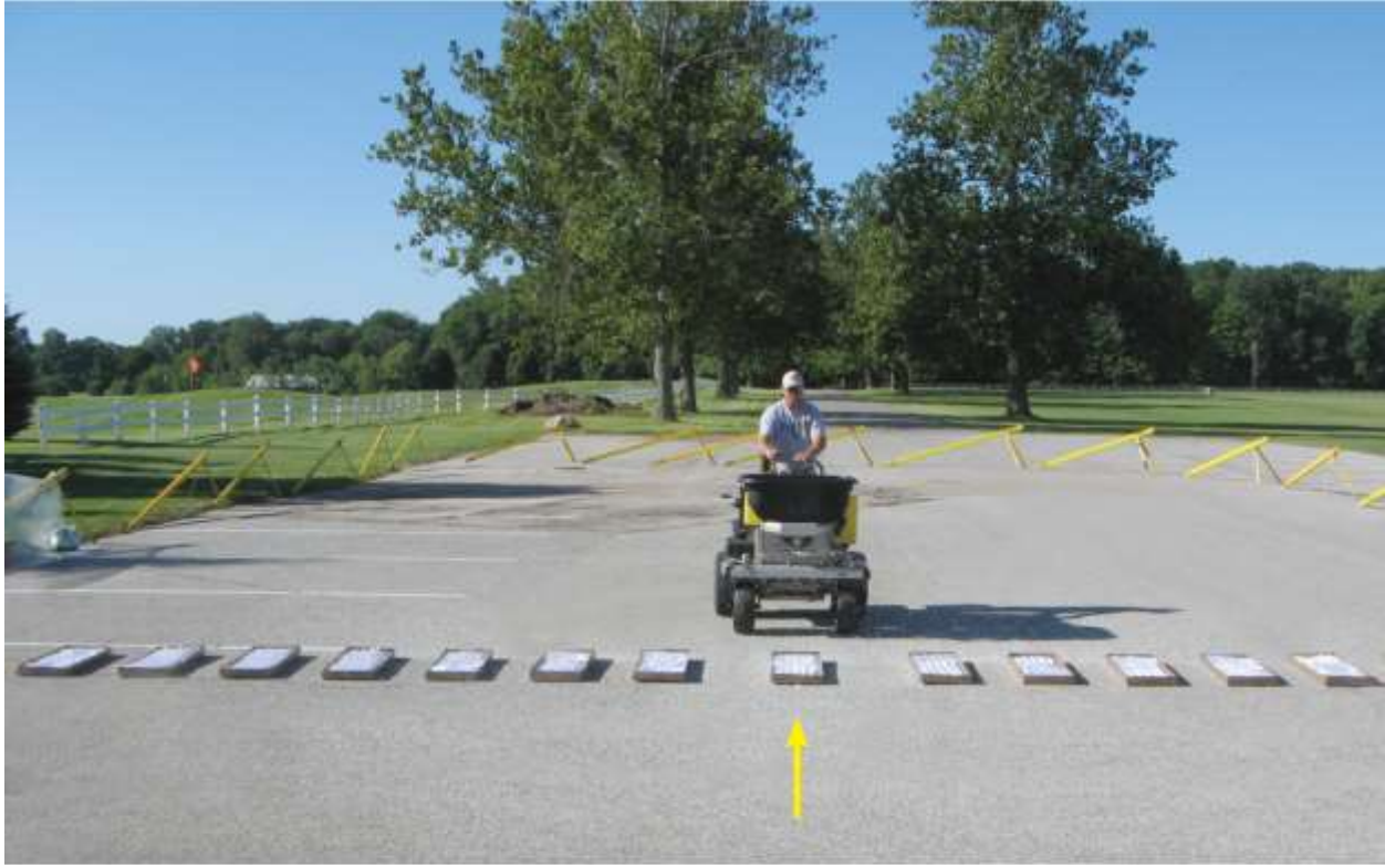
The center box is marked with an arrow. Notice the extra space on either side of the center box to allow room for the wheels. In this example, the spreader is being calibrated for a product with a large granule, so the boxes are placed about 12 inches apart to catch the granules along the entire width of the spread.
