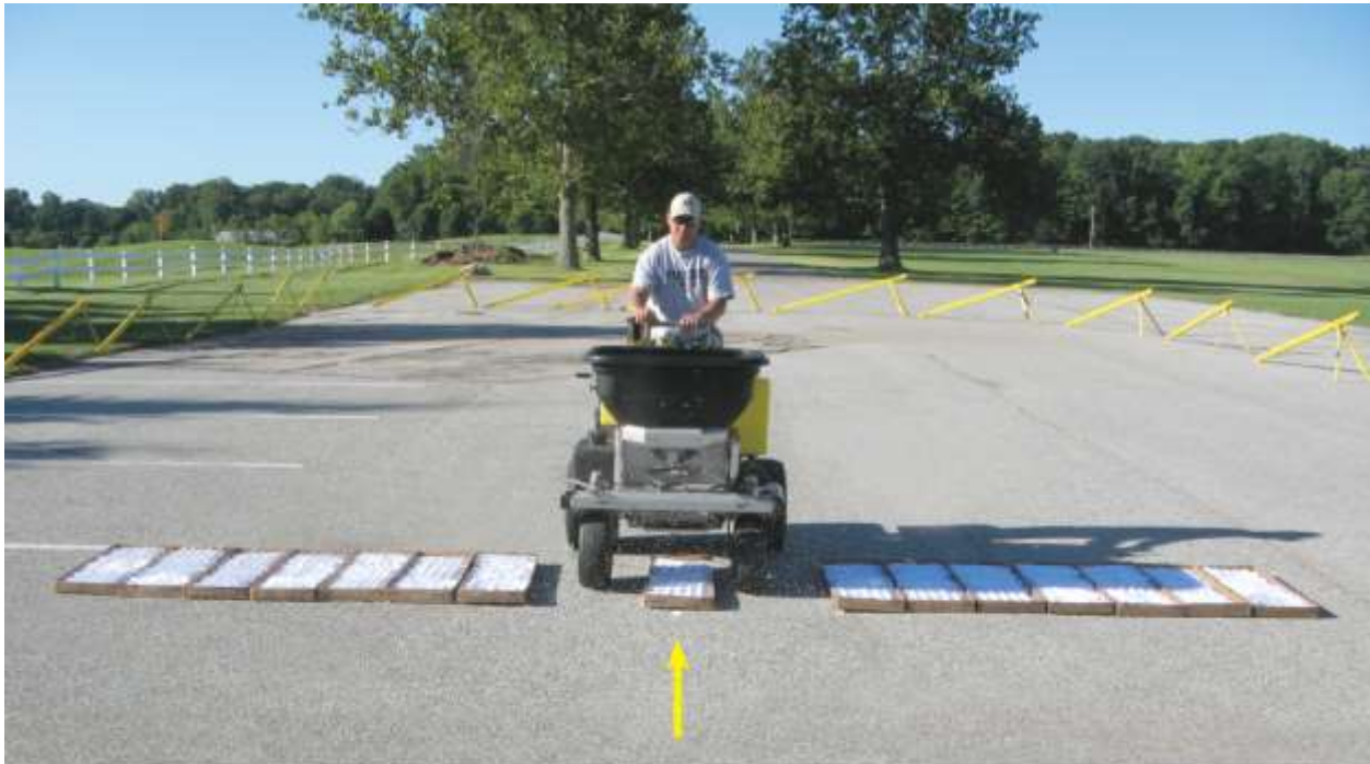
In this example, the spreader is being calibrated for a product with a small granule, so there is no space between the boxes. Closer box spacing with small granules helps you determine the effective spread width more accurately.
