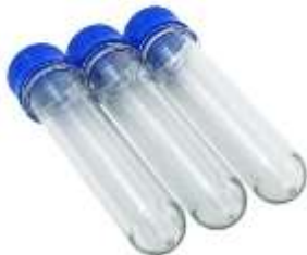
Figure 5. These Baby Soda Bottles (also known as Giant Test Tubes) can be ordered online. They hold 35 mL and work well for spreader calibration.
