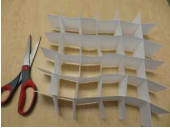
Figure 3. After making several pre-cut strips, fit the strips together using the slits to make baffles.
