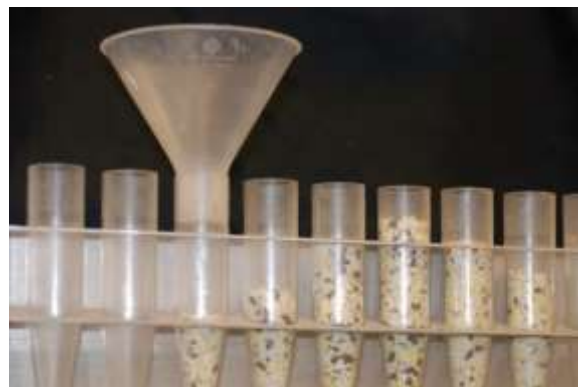
Figure 8. This test tube rack works well for displaying these tubes. A funnel is a helpful tool for pouring the fertilizer from the collection boxes into the tubes.
