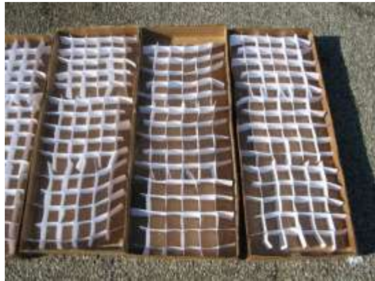
Figure 1. These custom 1 ft by 3 ft long collection boxes were made from cardboard scraps and packing tape.
