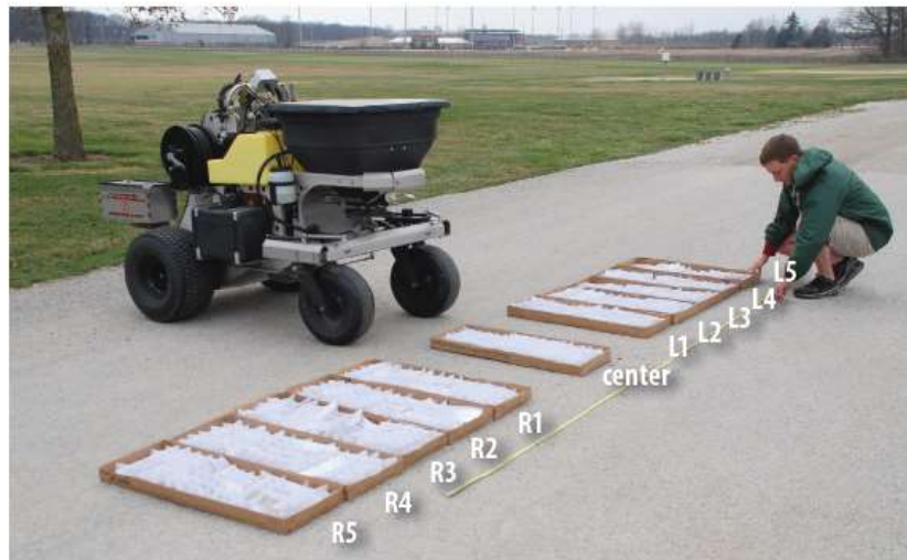
The effective spread width for this spreader is the distance from the box that corresponds to the L4 tube to the box that corresponds to the R4 tube.
