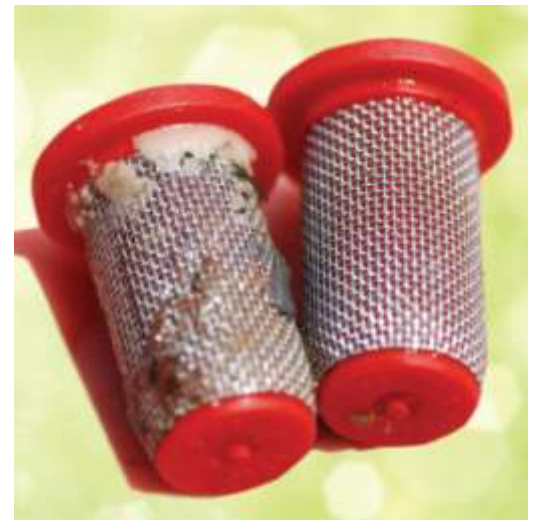
Something as simple as a partially clogged screen (left) can undermine any calibration by altering the flow of water. Clean screens (right) can help keep sprayer output consistent. Remember to clean any filters between the spray tanks and nozzles.
