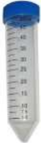
Figure 4. These plastic 50 mL centrifuge tubes are one option as a type of tube that can be used for spreader calibration.
