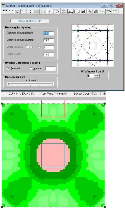
The square design at head-to-head spacing has a CU of only 84% and DU of 75%. We can do much better. The Scheduling Coefficient, by the way, of 1.4, indicates that the system would need to run 40% longer compared to if the CU was 100%; so there is a wastage factor of 40%. Using a triangular design with the laterals brought in 3m, as shown below, the Densogram on the next page looks a lot better:
