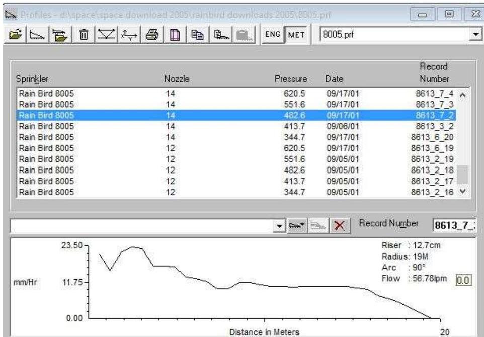
We could then set up the 8005 heads on a square design at head-to-head spacing, as below, and model the result as a Densogram (over the page):
