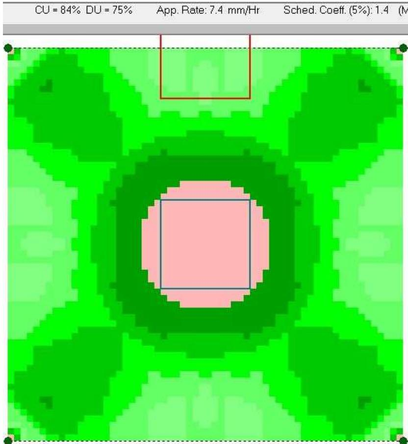
The square design at head-to-head spacing has a CU of only 84% and DU of 75%. We can do much better. The Scheduling Coefficient, by the way, of 1.4, indicates that the system would need to run 40% longer compared to if the CU was 100%; so there is a wastage factor of 40%. Using a triangular design with the laterals brought in 3m, as shown below, the Densogram on the next page looks a lot better:
