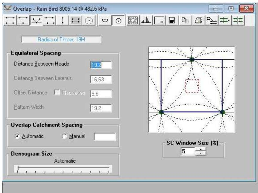
Densogram on a triangular design at 19.2 head spacing, 16.6m lateral spacing. Note the CU, DU and SC figures now. The figures can be improved even further, and the SPACE program lets you model several configurations. Putting the irrigation heads at 15m spacing, for example, results in very high CU values, but cost would become an issue.
